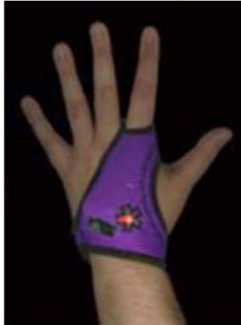
Figure 2. The Galvactivator, a glove-like instrument that measures the wearer's skin conductivity [18].
