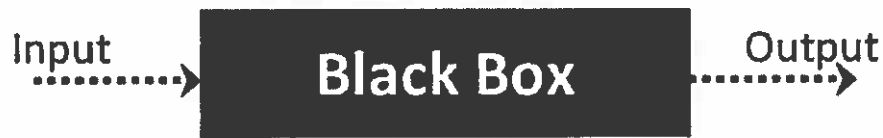
Figure 13 [16]: A representation of the basis of a black box testing. The 'Black Box' is where the code is and has abstraction, thus, we do not see the code.
