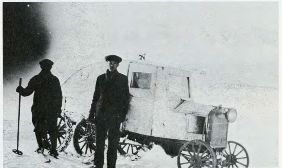
Snowmobile made from a Model T Ford, 1930, by Alfred Wilson and Austin Greenway.
