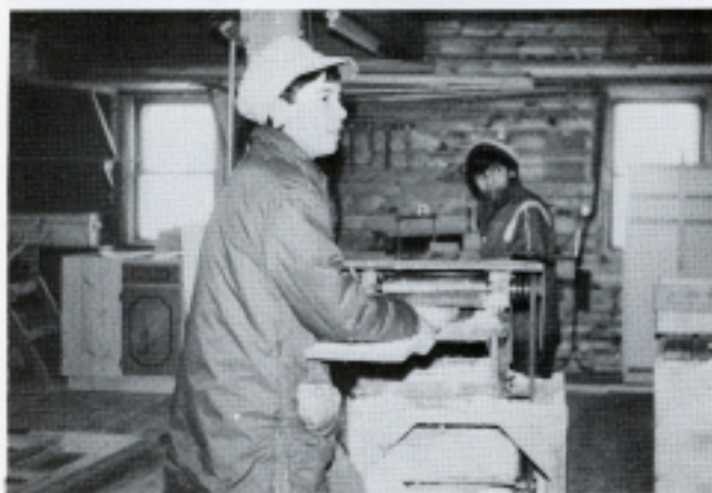
We stack the boards first so they will dry. Then we plane them to make them smooth. We use the boards for making cabinets. Clifford
