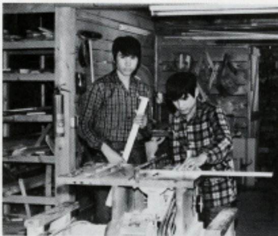
We use the power saw to cut our boards into the right width. Keep your fingers at least four inches away from the blade. Steven
