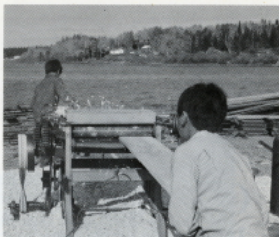
We planed the boards for our house because they are not the same thickness and because they are rough. Richard
