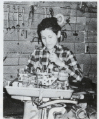
Checking breaker point gap.
