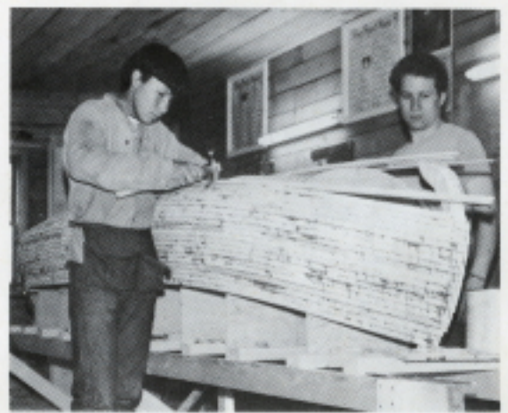
Our 16-foot canoe has 1/4" x 3/4" spruce wood strips. They are glued and nailed to plywood forms. We put fiberglass on both sides. Ernest
