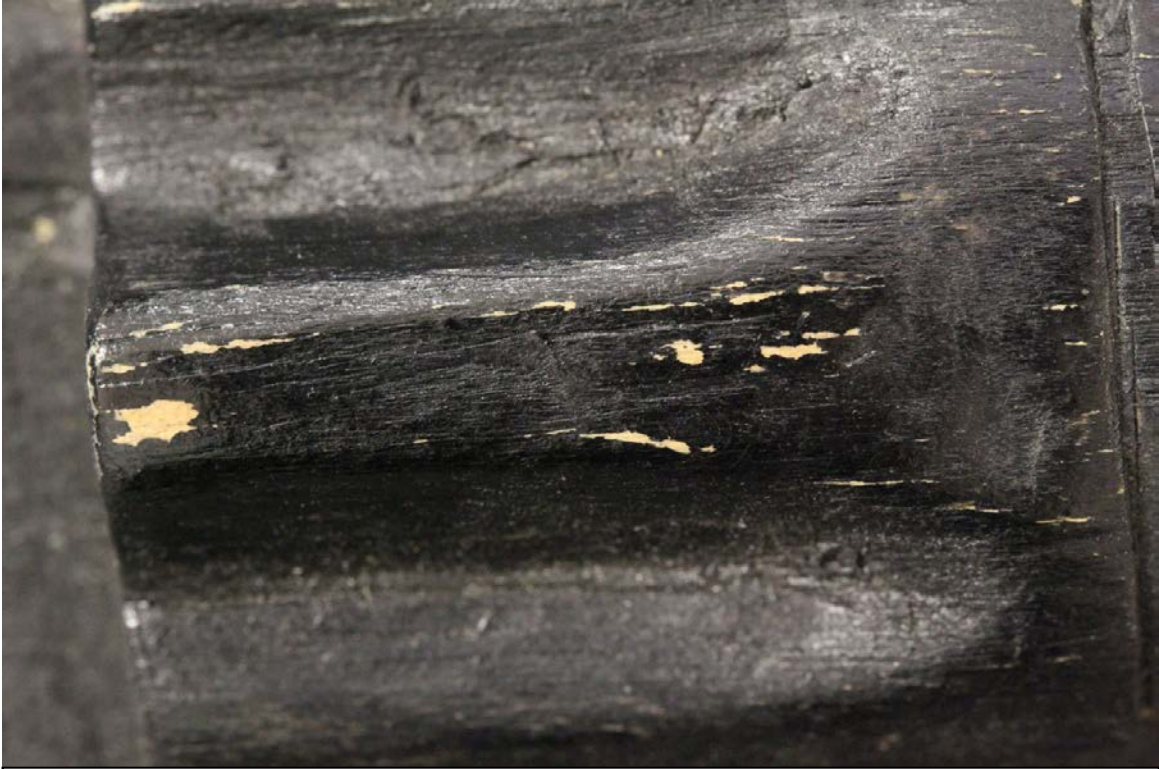
Fig.3 – Chipping – Right center
