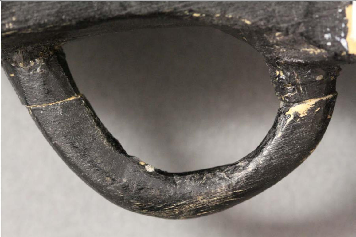
Fig.4 – Chipping – Right center
