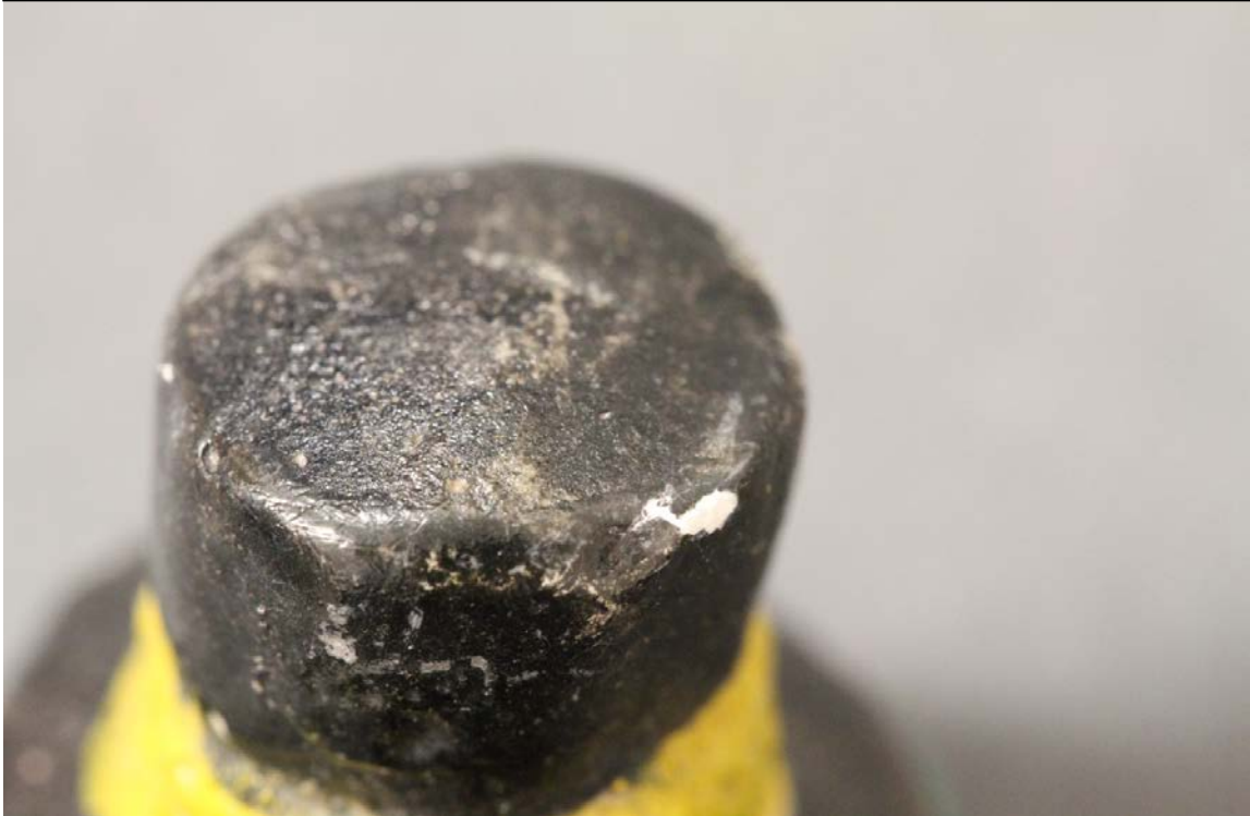
Fig.4 – Chipping – Back top
