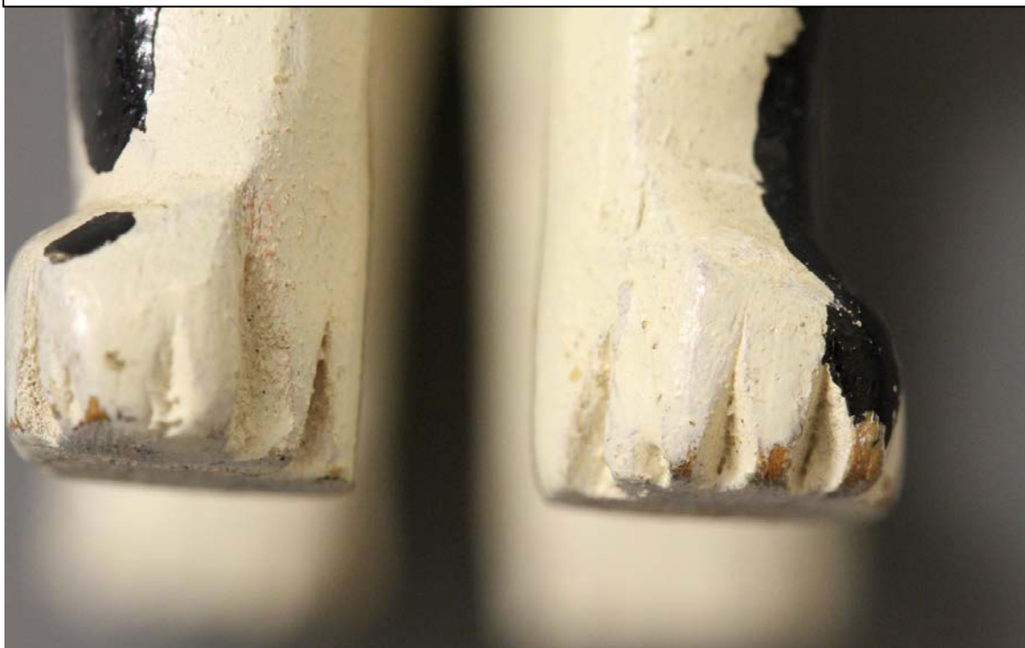
Fig.2 – Wear – Front bottom edge
