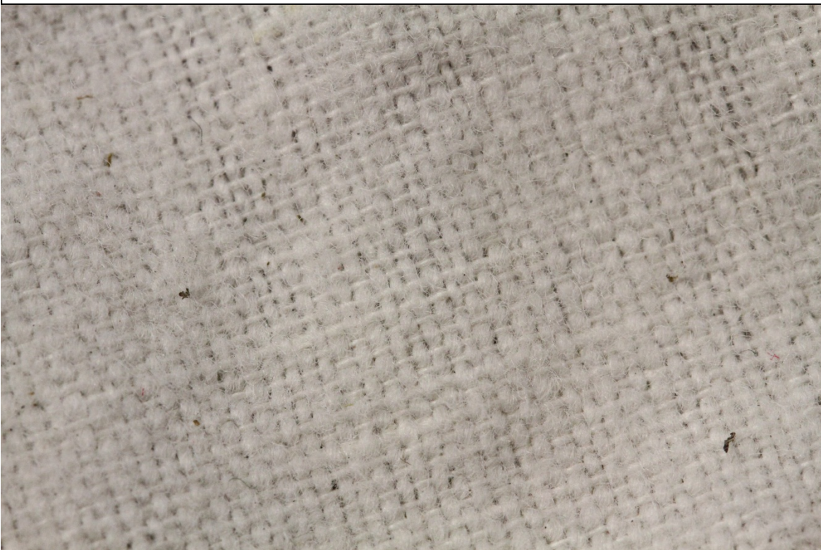
Fig.4 – Discolouration – Inside layers
