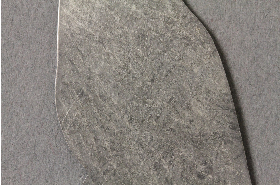
Fig.1 – Corrosion – Front center
