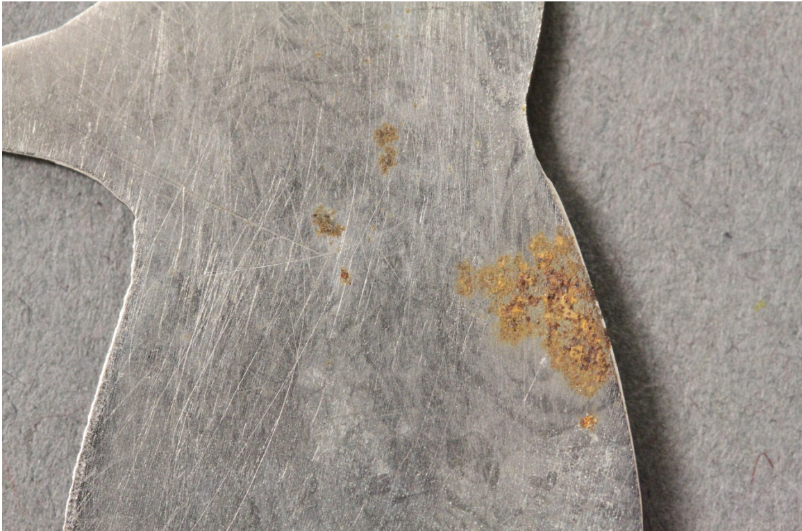
Fig.1 – Corrosion – Front top right
